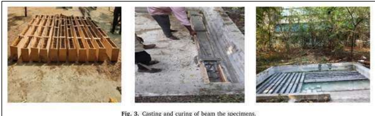
Fig. 3. Casting and curing of beam the specimens.
