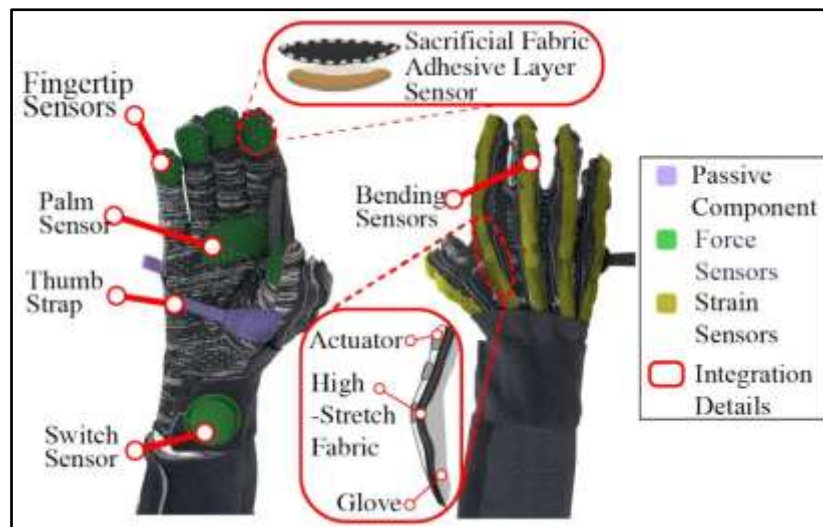
Figure 4. Highlighted sensors and a passive component with integration details illustrated in an integrated glove [43].
